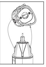
• To attach a head, align the slots on the head with the ribs on both sides of the trimmer unit as shown below, until it meets the magnet and is securely held in place.
