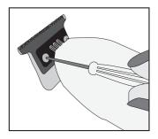
**Step 5.** Remove the zero gap tool from the blade by pushing it gently down.
