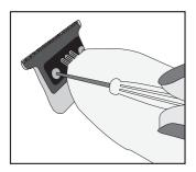
**Step 2.** Place the zero gap tool on to the bottom of the blade.
