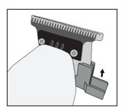
**IMPORTANT!** Be sure the blades are aligned properly. The teeth of the smaller blade (cutter) should rest slightly below the upper edge of the larger blade.
