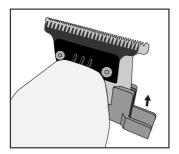
**IMPORTANT!** Be sure the blades are aligned properly. The teeth of the smaller blade (cutter) should rest slightly below the upper edge of the larger blade.
